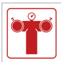
Fire pump connection
