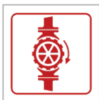
Sprinkler stop valve
