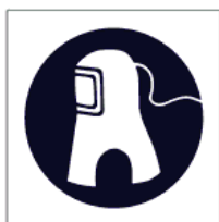
Air-supplied hood shall be worn
