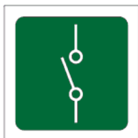
Electric isolator switch
